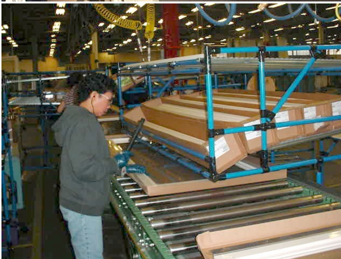
Workstations on the main assembly line were redesigned to place parts within easy reach in front of operators.
