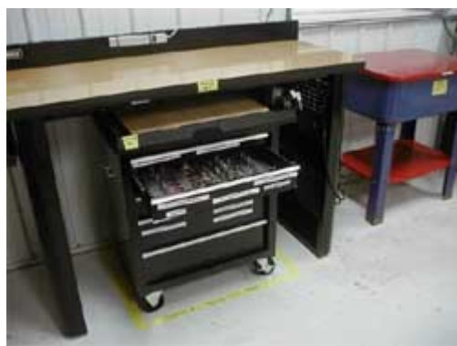
The mechanic in dealership (same as pictured at top) found himself wiggling into a too-tight space to use the red and blue worktable in this picture. After 5S, the table was moved to a more suitable location, the tool chest was labeled and tucked away to save floor space, and areas of the floor were labeled with yellow tape to mark off boundaries. Now, the mechanic and his colleagues are able to find and use tools easily without everything spreading around the space at the risk of being damaged or misplaced. All photos: Ariens.
