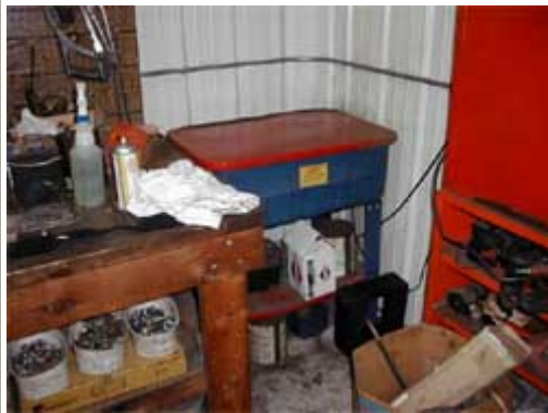
The mechanic in dealership (same as pictured at top) found himself wiggling into a too-tight space to use the red and blue worktable in this picture. After 5S, the table was moved to a more suitable location, the tool chest was labeled and tucked away to save floor space, and areas of the floor were labeled with yellow tape to mark off boundaries. Now, the mechanic and his colleagues are able to find and use tools easily without everything spreading around the space at the risk of being damaged or misplaced. All photos: Ariens.
