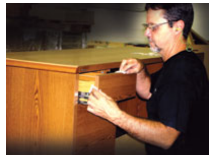
Scott Dingler, utility lead, cycle tests a drawer on a wooden desk and prepares to install packaging foam.
