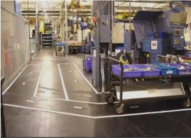
FIFO lanes at the spindle and cuff cell control the mix and flow of parts across machines. Each blue bin on the cart contains a spindle or cuff for processing.
