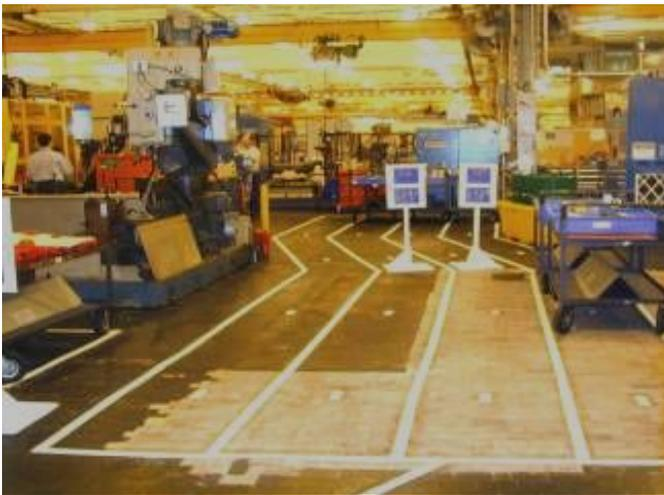
Signposts in FIFO lanes at the spindle and cuff cell show operators the next operation for each part.
